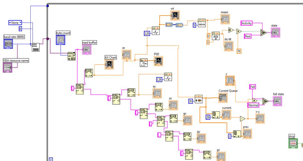
Figure.4. Screen Shot of Lab view Block diagram for detection of Seizure
