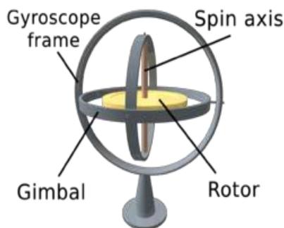
Figure.2.Gyroscope with freedom in 3 axes
