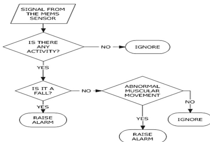
Figure.3. Flowchart for detection of Abnormal signals
