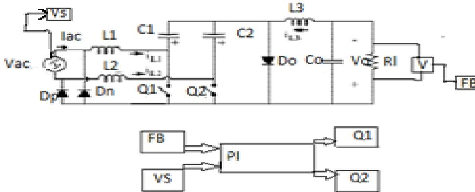
**Fig.5. Bridgeless rectifier with PI controller**
