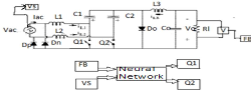
**Fig.9.A Bridgeless Rectifier with Neural Network of CUK Converter**
