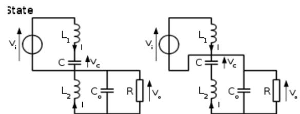
Fig.2.CUK Converter operation
