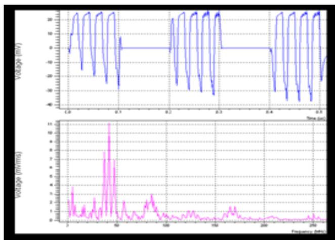
**Figure.4. Output pulses generated through Resistive sensing UWB pulse generator**
