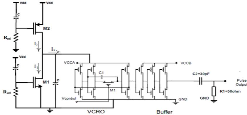
**Figure.6.Capacitive Sensing UWB pulse generator**
