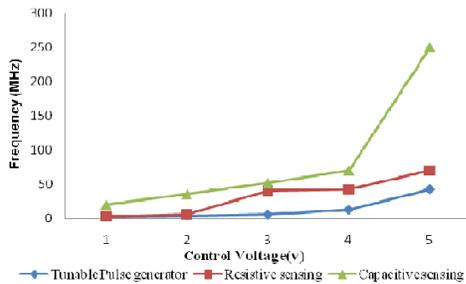
Fig.8. Pulse frequency Vs control voltage characteristics
