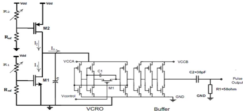
**Figure.3.Resistive sensing UWB pulse generator**
