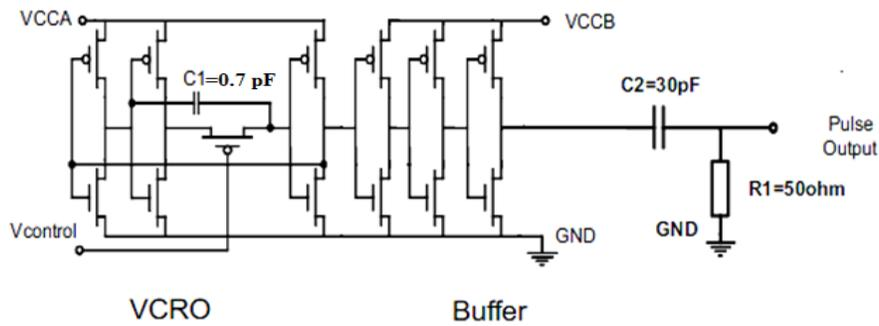
**Figure.2.Tunable pulse generator**
