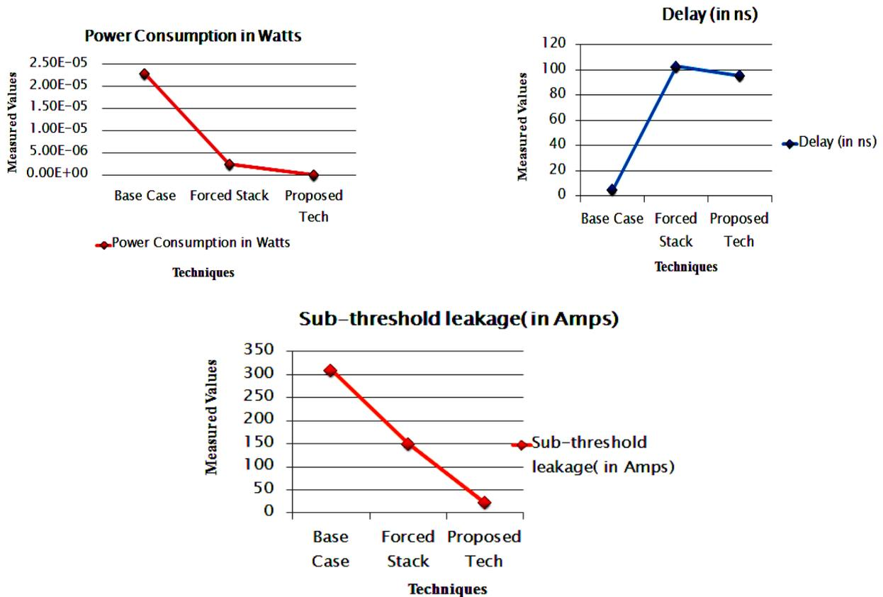
**Fig.5. Illuminates the amount of power consumed, delay and Sub-threshold leakage existing technique at the 45nm technology in active and standby modes**
