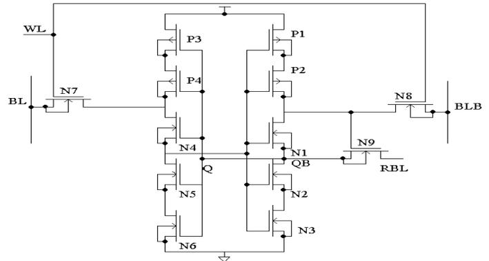
Fig.2. Forced Transistor Stacking
