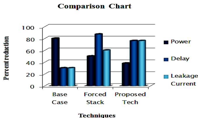
**Fig.6. Illuminates the comparison chart of power, delay and Sub threshold leakage in active and standby modes**
