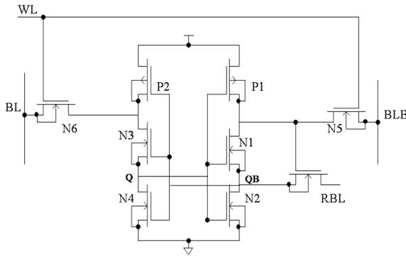
Fig.1. Conventional 9T SRAM
