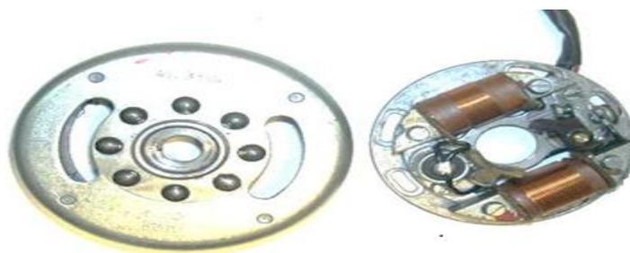
Figure.3.Magneto ignition system
