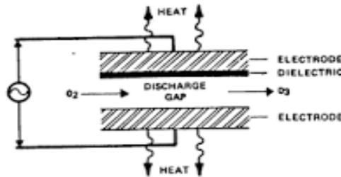
Fig.1.DBD equivalent circuit
