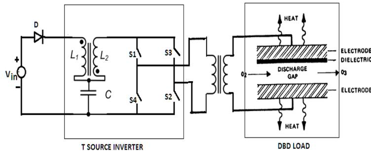
Fig.2.T source inverter with DBD load
