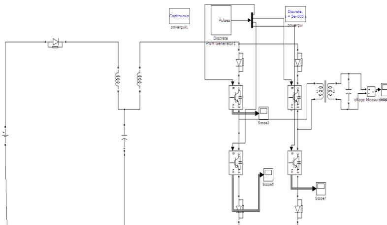
**Fig.5.Simulation diagram of TSI with DBD load**
