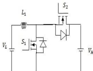
Fig.1. Conventional bidirectional converter
