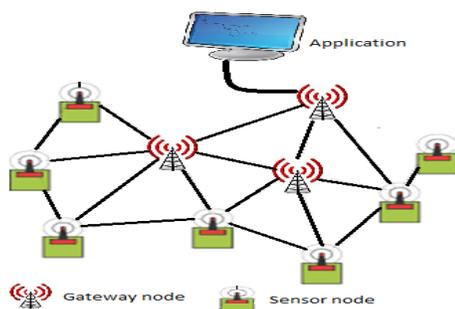
Fig.1.Block diagram of Wireless Sensor Network
