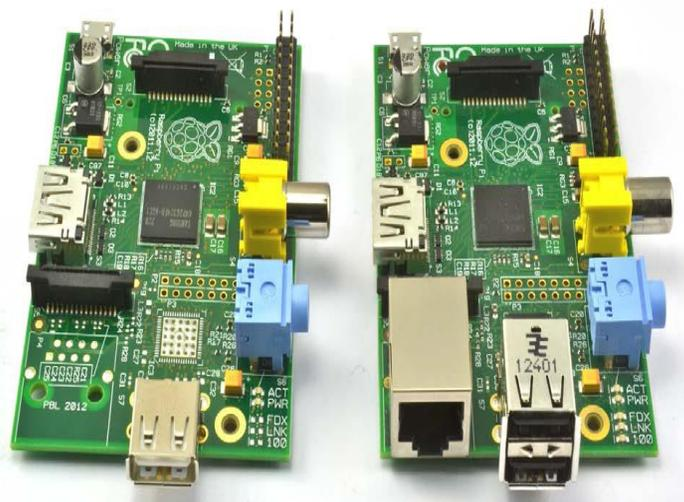
**Figure.5. Raspberry pi Microcontroller**
