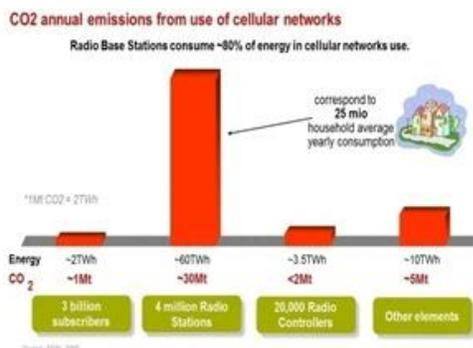
Fig.1. CO<sub>2</sub> emission from use of cellular networks
