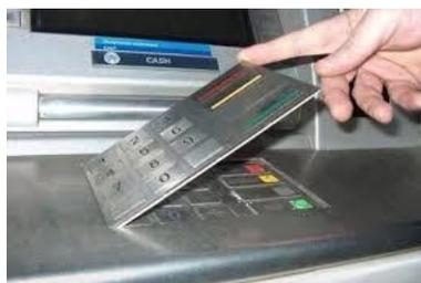
**Fig.2. Card reading keyboard to enter pin**
