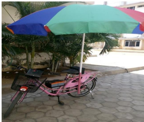
Figure.4. Photograph of Proposed PV based Bicycle
