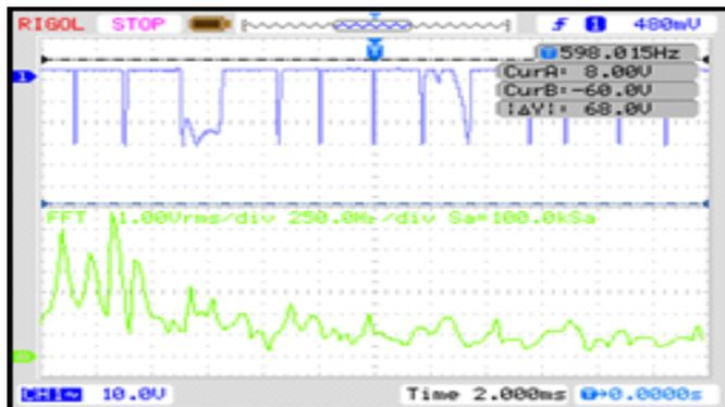
**Fig.5.Neutral Current Harmonics Without Filters**
