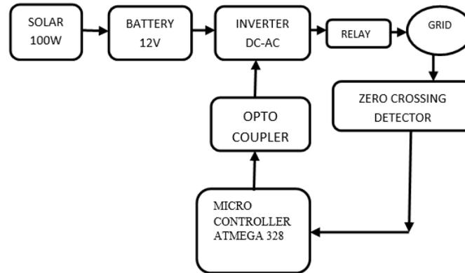
**Fig.1. Block diagram using grid tie inverter**
