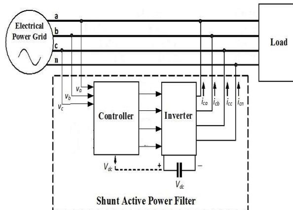
**Fig.2. Block Diagram of Shunt Active Filter**
