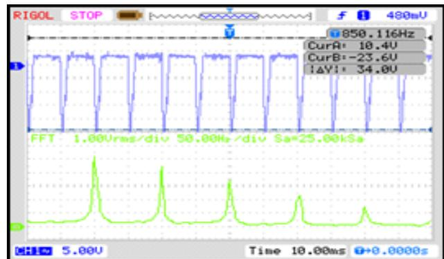
**Fig.6.Neutral Current Harmonics With Filters**
