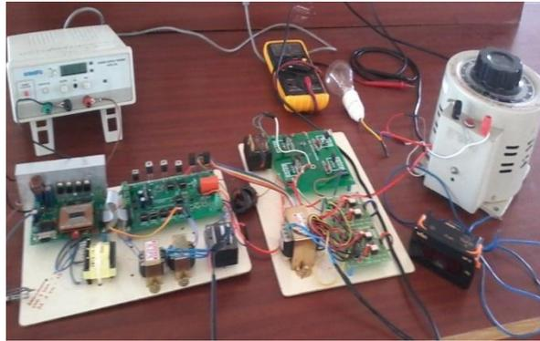
**Fig.4.Hardware Model- Grid Tie Inverter**
