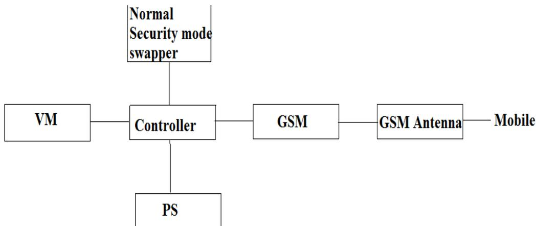
**Fig.4. Block Diagram of GSM based voting system**
