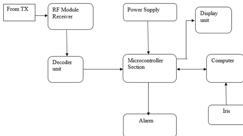
**Fi.6. Block diagram of Receiver Section**
