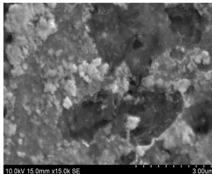
Figure 4: SEM image of CuO nanoparticles
