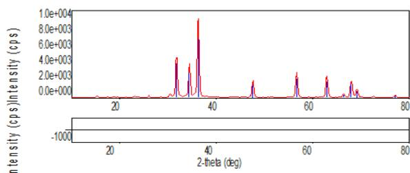
Figure1: Wide angle XRD patterns of ZnO nanoparticles calcined at 400°C
