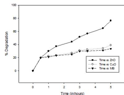
Fig 5. Comparison of the photocatalytic activities of the ZnO and CuO nanoparticles
