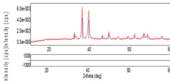
Figure 2: Wide angle XRD patterns of CuO nanoparticles
