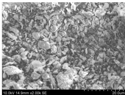
Figure 3: SEM image of ZnO nanoparticles
