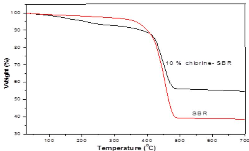
**Figure.3. Thermal degradation curve of SBR and functional group introduced SBR**
