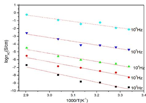
Figure.6.Variation of  $\log \sigma_{AC}$  ( $\sigma_{AC}$  in S/cm) with  $1000/T$  ( $K^{-1}$ ) of 5% Cl sample
