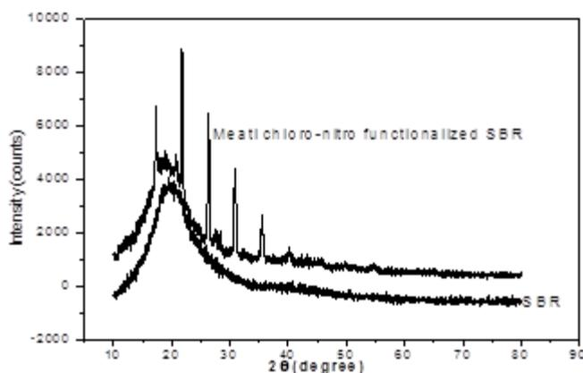
**Figure.1.XRD patterns of SBR and chemically modified SBR**
