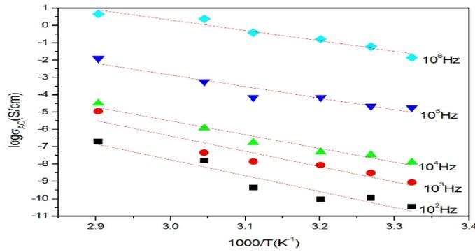
Figure.7.Variation of  $\log \sigma_{AC}$  ( $\sigma_{AC}$  in S/cm) with  $1000/T$  ( $K^{-1}$ ) of 10% Cl sample
