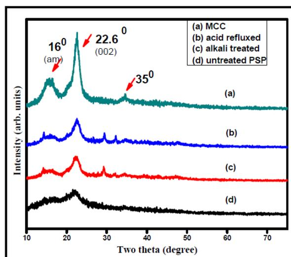
Figure.4. XRD patterns of (a) MCC (b) acid refluxed (c) alkali treated (d) untreated PSP
