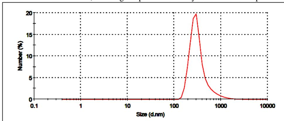
Fig.5. Size distribution of freeze dried cellulose samples by number
