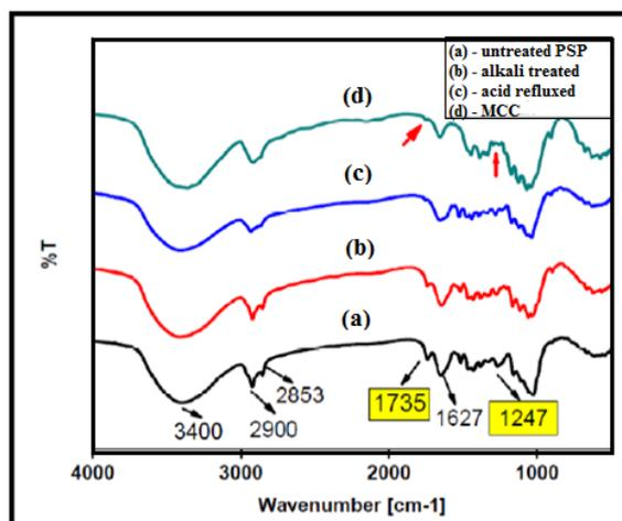
Fig.3. FTIR spectra of (a) untreated PSP (b) alkali treated (c) acid refluxed (d) MCC
