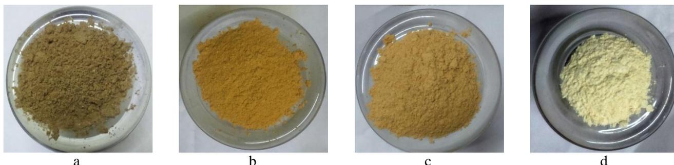
**Fig.1. Photographs of (a) pure PSP (b) alkali treated (c) HNO<sub>3</sub>/ ethanol refluxed (d) MCC**
