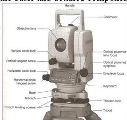
Figure.5. Total Station Parts an Overview
