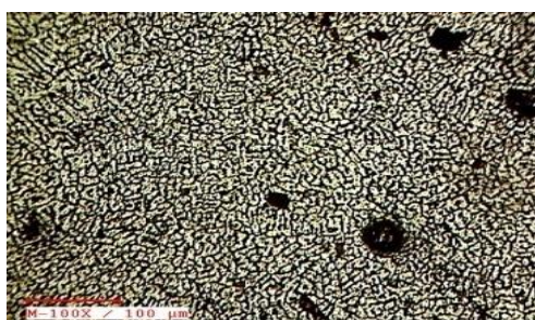
Figure.3. Weld at Middle ER4043
