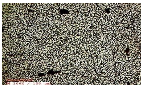
Figure.5. Weld at Bottom ER4043
