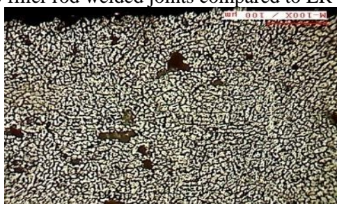
Figure.1. Weld at Top ER4043
