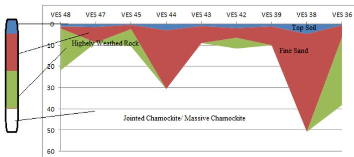
Figure.6. Geophysical survey locations with cross section map
