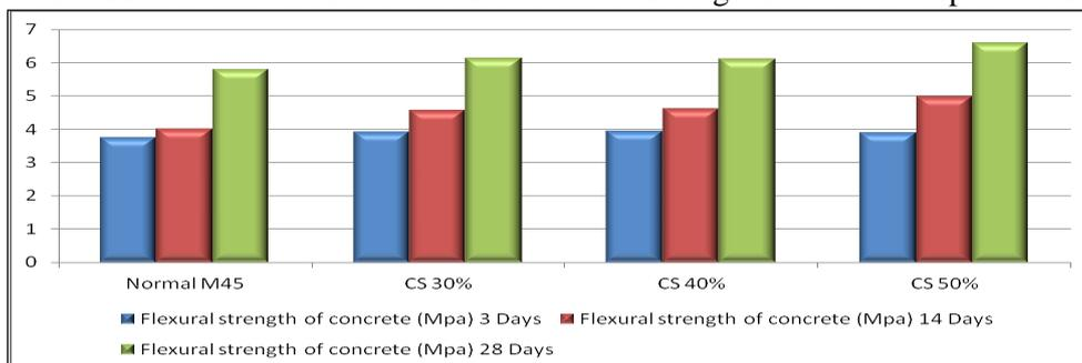
**Figure.7.Flexural strength variation different mix proportions**
