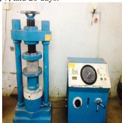
**Figure.4.Compression test on concrete cube**
