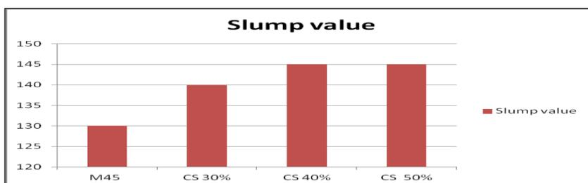
**Figure.3.Slump value for different mix proportions**
