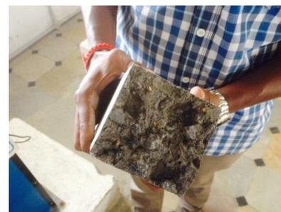
**Figure.5.Flexural test on concrete beam**
