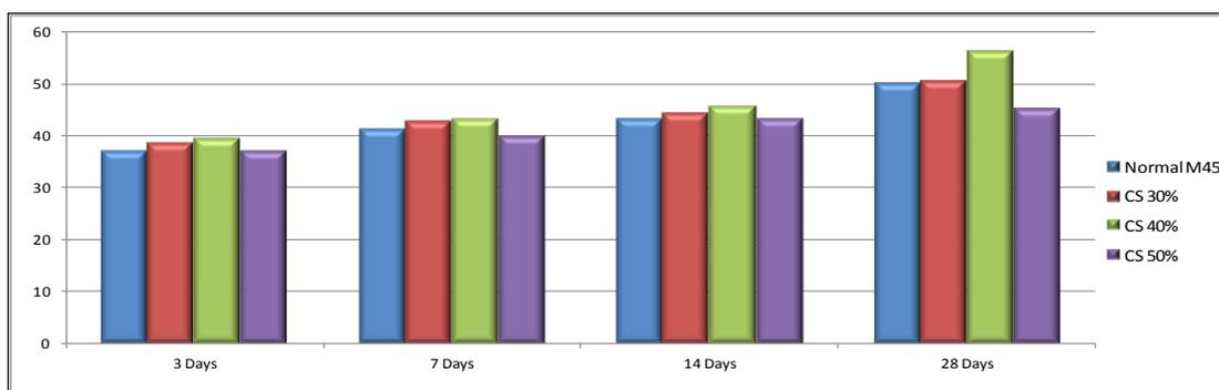
**Figure.6.Compressive strength variation of different mix proportions**
