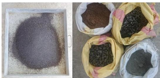
Figure.1. Copper slag, Sand, Coarse aggregate and fine aggregates
