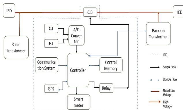
Fig. 2 Block Diagram of Transformer Attached IED
