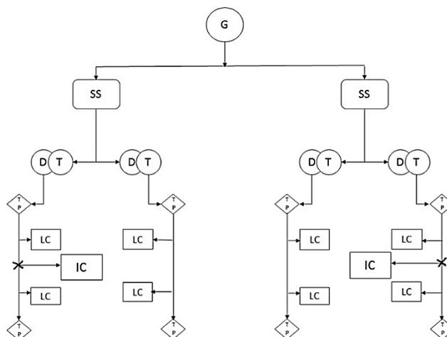
**Figure.4.IED Interfaced Layout of Smart Grid System**
