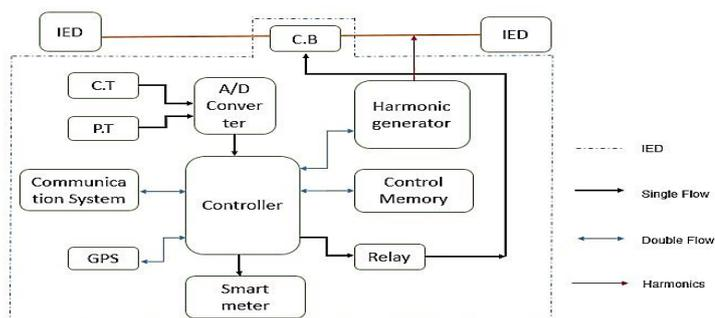
Figure.1. Block Diagram of Pole Attached IED
