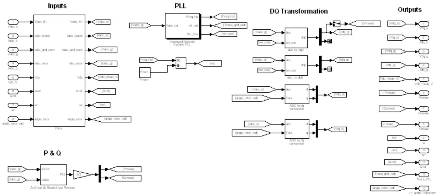
Fig.1 MATLAB simulation of (PMSG) wind turbine with dq-transformation and phase lock loop (PLL)
