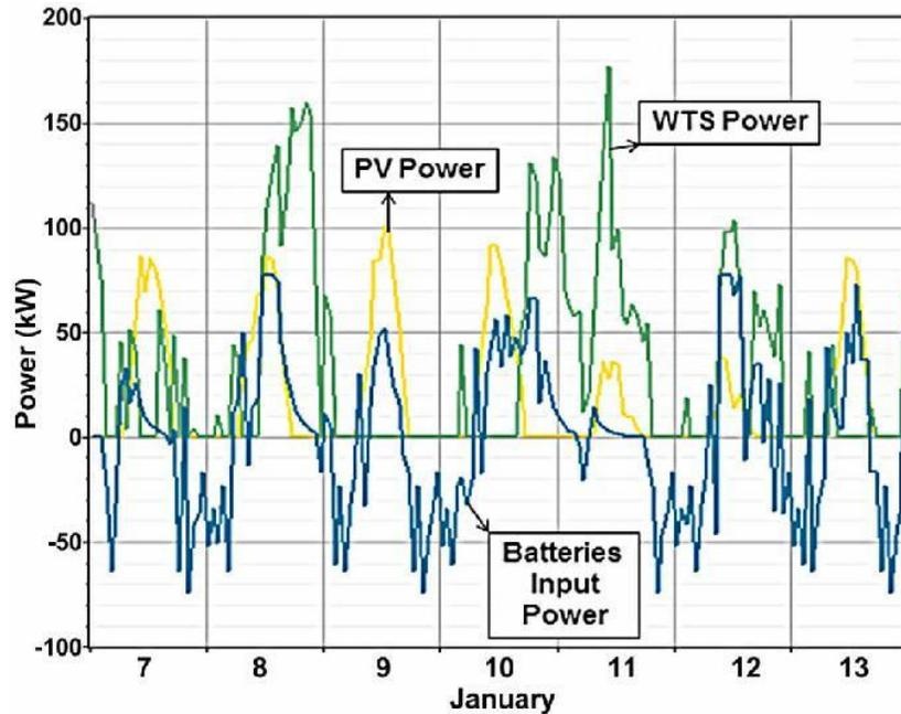
Figure.2.Power contribution by individual sources and battery bank
