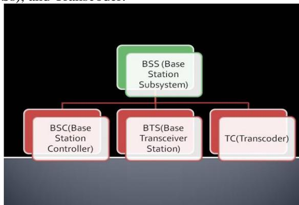
Figure.5. Block Diagram of Base Station System
