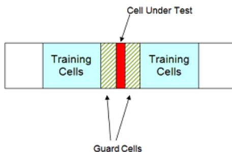
**Figure.3.CFAR Test Cells**
