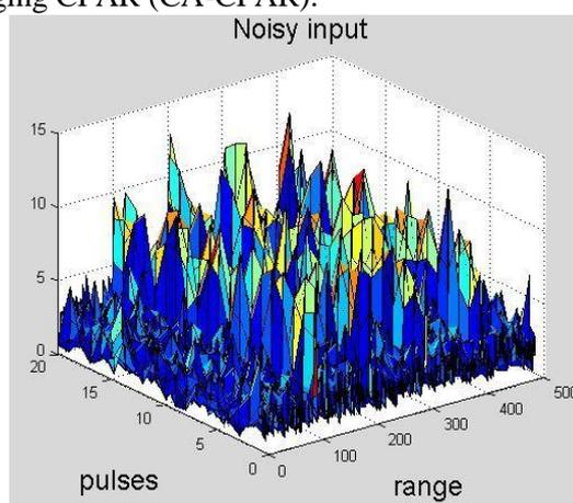
**Figure.11. Targets Suppressed by clutter**
