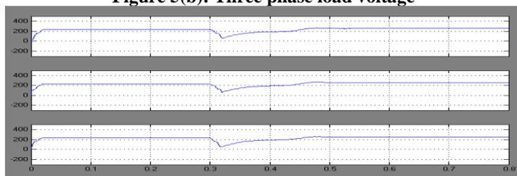
**Figure 5.2: Three phase load voltage (RMS)**
