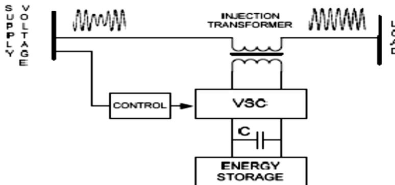
Figure.1. Typical DVR circuit topology (Single-phase representation)
