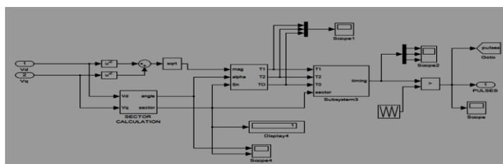
Figure 4(b): Control Block Diagram of SVM implemented
