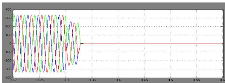
Figure 5(a): Three phase fault (Load voltage with fault conditions)
