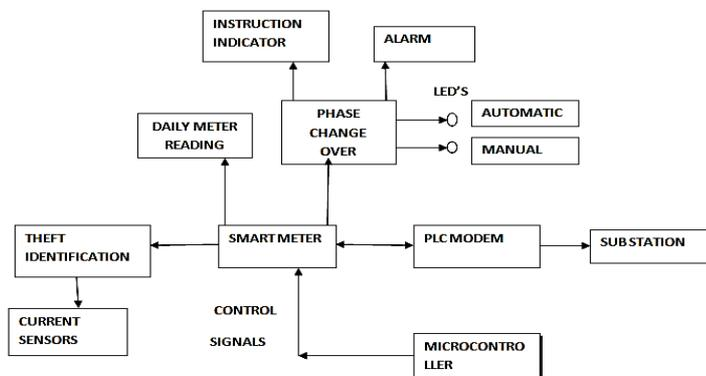
**Figure.1. Block Diagram of smart meter controller**
