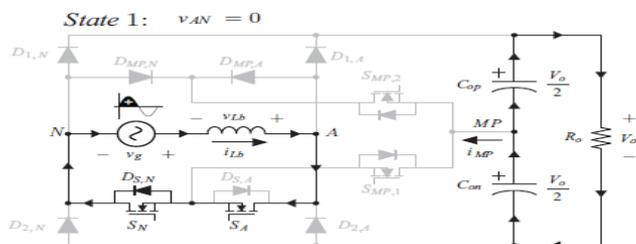
**Figure.3. Mode 1 operation of the proposed circuit**
