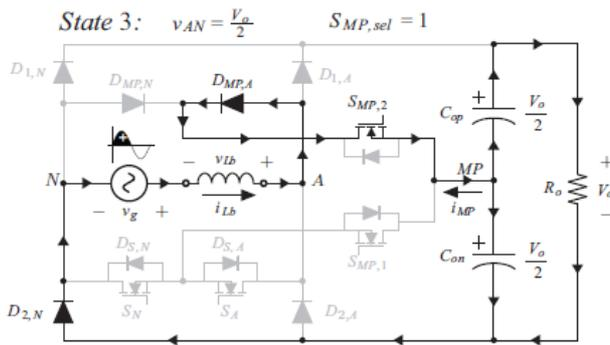
**Figure.5. Mode 3 operation of the proposed circuit**
