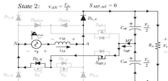
**Figure.4. Mode 2 operation of the proposed circuit**
