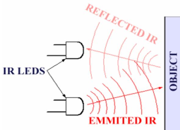
Figure.6.Working of IR sensor
