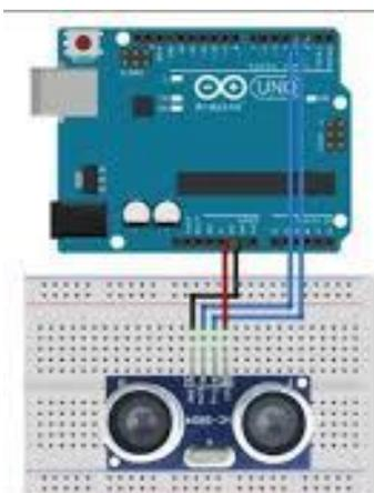
**Figure.11.Arduino output of Ultrasonic Sensor**
