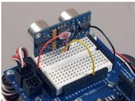
**Figure.9.Wiring diagram of Ultrasonic sensor**
