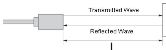
**Figure.3.Basic working of ultrasonic sensor**
