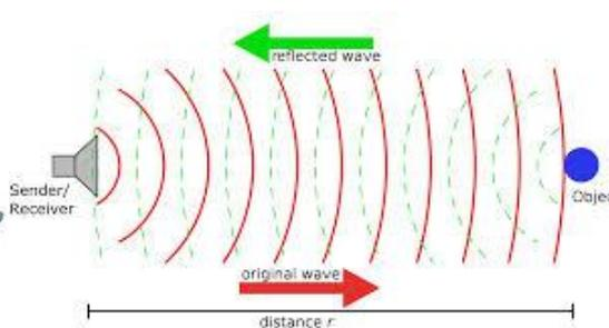
**Figure.5.Working of the Ultrasonic sensor**
