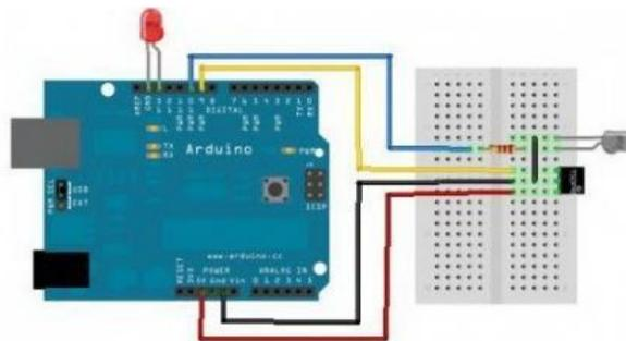
**Figure 10 Wiring diagram of IR Sensor**
