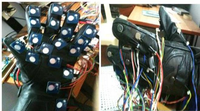
**Figure.3. The hardware prototype of the glove**
