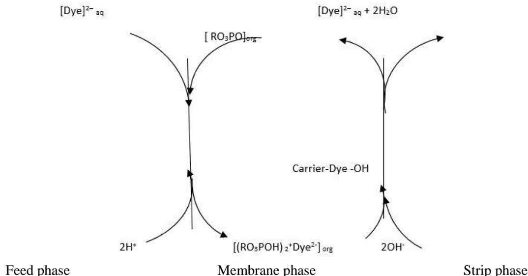
**Figure.6. Schematic Representation for Transport of Anionic Dyes by Supported Liquid Membrane**
