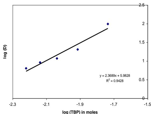
**Figure.4.Relationship between log D and log (TBP) for Acid Red 10B**
