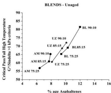
**Figure 4(a) Asphaltenes Vs. High Temperature (HT) For Rut Resistance**
