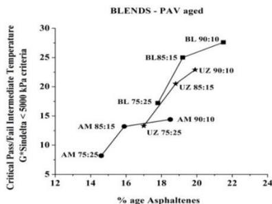
**Figure 4(b) Asphaltenes Vs. Intermediate Temperature (IT) For Fatigue Cracking Resistance**
