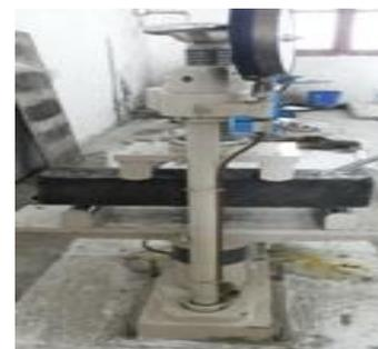
Fig.9.Flexural Test of Beams
