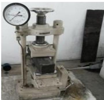
Fig.8.Flexural Test of Beams
