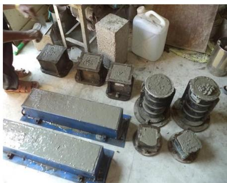
**Fig.2.Batching of Concrete**
