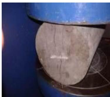
Fig.7.Split Tensile Test in CTM
