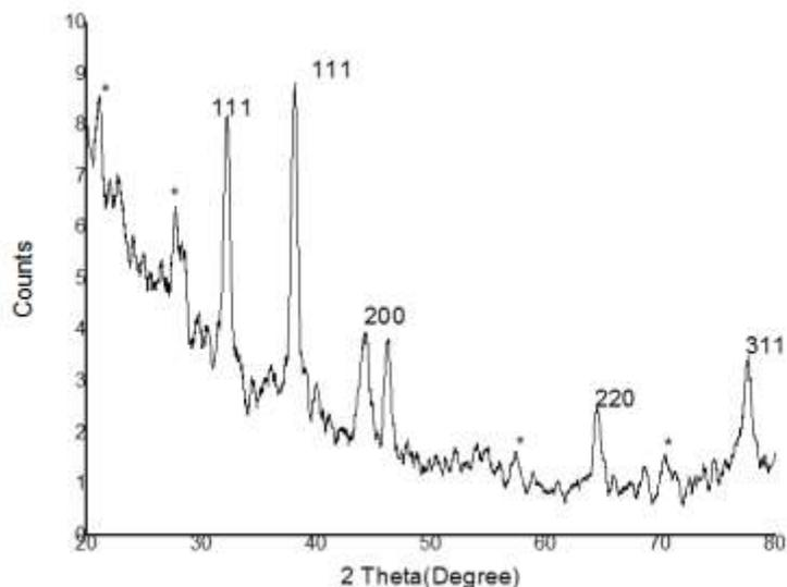
**Figure 3, XRD pattern of biosynthesized silver nanoparticles**
