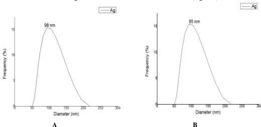
**Figure 2, Particle size analyse in DLS mode using zeta size A – Aqueous Sample; B – Dry Sample**
