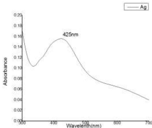
**Figure 1, UV-Visible spectra of Ag nanoparticles**
