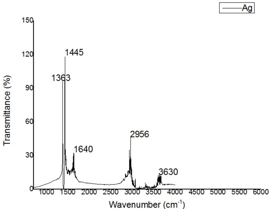
Figure 2, FTIR Spectra of the synthesized particles
