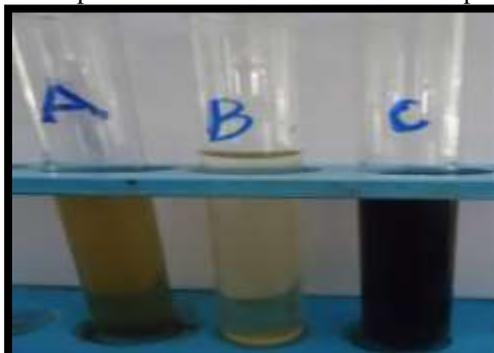
Fig.1 Visual observations of A - Leaf extract, B - Ferrous Sulphate and C- Iron oxide Nanoparticles
