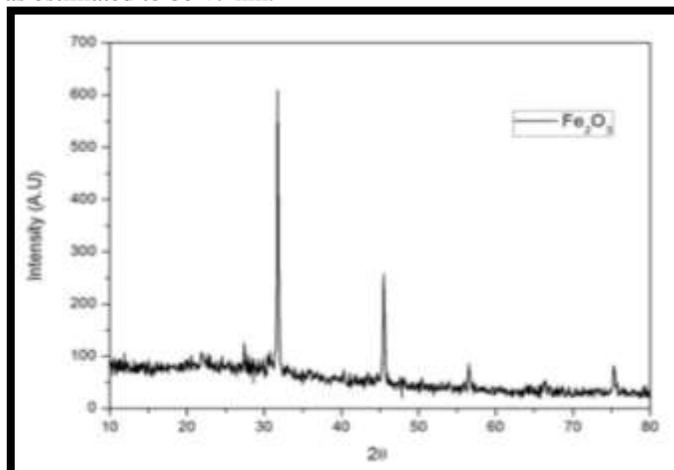
Fig.4 XRD pattern of synthesized iron oxide nanoparticles
