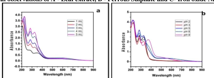
Fig. 2 (a) UV-Visible spectra of iron oxide nanoparticles at 1 mM ferrous sulphate with different volume of extract, (b) UV-visible spectra of iron oxide nanoparticles at different pH
