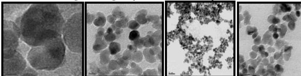
Fig.6 TEM images of synthesized iron oxide nanoparticles
